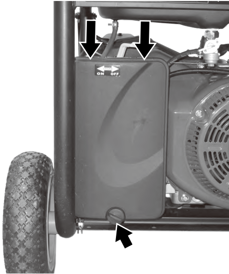
Installation of Air Cleaner Cover
