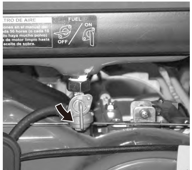
Fuel Shutoff Valve in the ON Position
