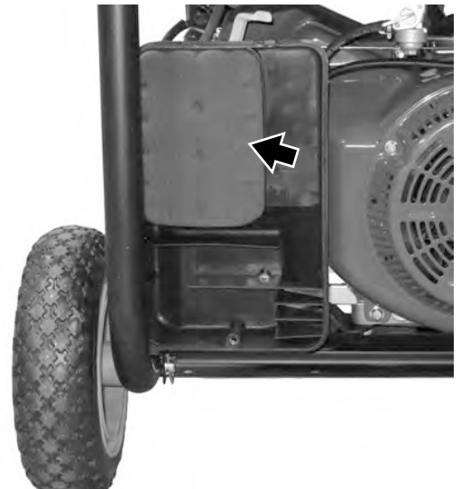
Removing Air Filter Element
