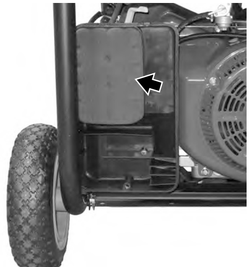
Removing Air Filter Element
