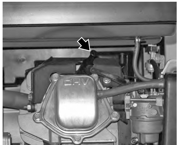
Removal of Spark Plug Boot
