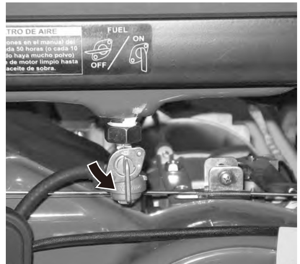
Fuel Shutoff Valve in the ON Position
